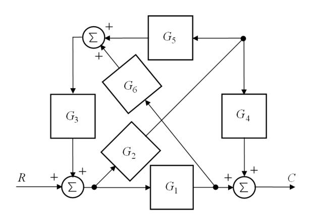
Moving  $G_2$  forward into the two branches enables us to combine the two nodes indicated.
