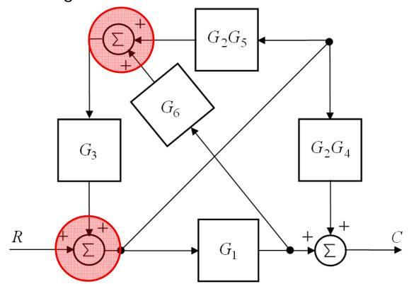
$G_3$  has been moved backward into the two branches enabling us to combine the two summing nodes indicated.
