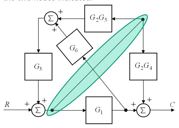
Moving  $G_3$  backward into the two branches enables us to combine the two summing nodes indicated.
