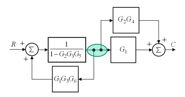
Notice that the block on the left is in standard feedback form and the block on the right comprises two parallel system blocks.
