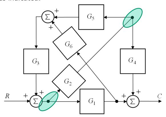
$G_2$  has been moved forward into the two branches enabling us to combine the two nodes indicated.
