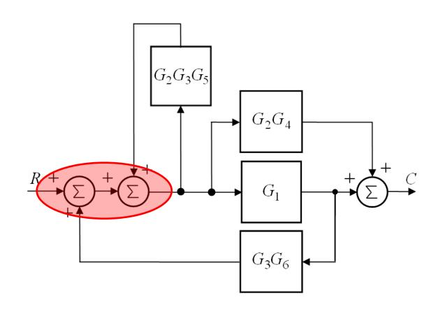
We recognize the indicated block as being in standard feedback form.
